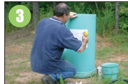
3 Use 1/2" drill bit to drill a saw starter hole at the location marked on the template.
