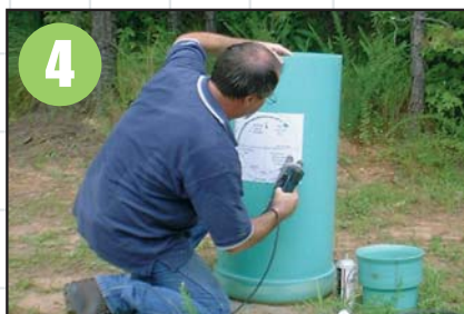
4 Use a jigsaw to cut between the marked lines (follow the lines carefully). Remove burrs with a file or knife.
